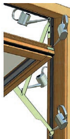
Figure 7.10. Lubricating a top swing gearing
