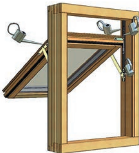
Figure 7.7. Lubricating a top guided gearing
