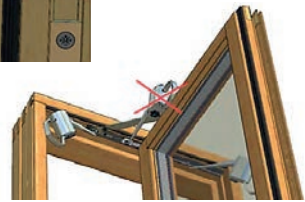
Figure 7.6. Lubricating a side projecting gearing
