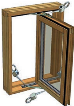
Figure 7.4. Lubricating side projecting gearing
